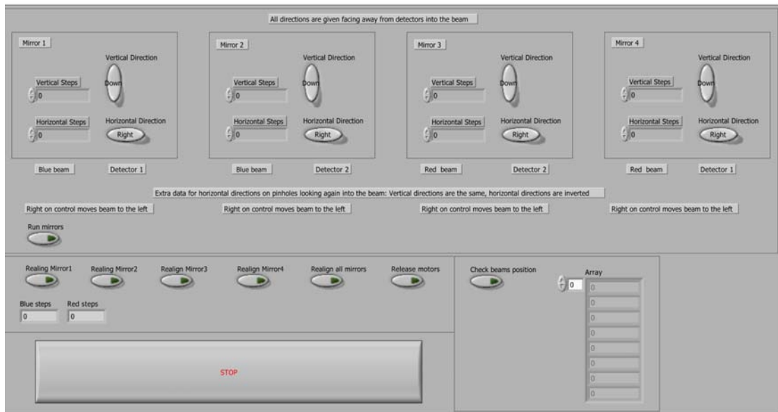
Figure G.4. Front panel of the VI for manual alignment of the computer-controlled mirrors
